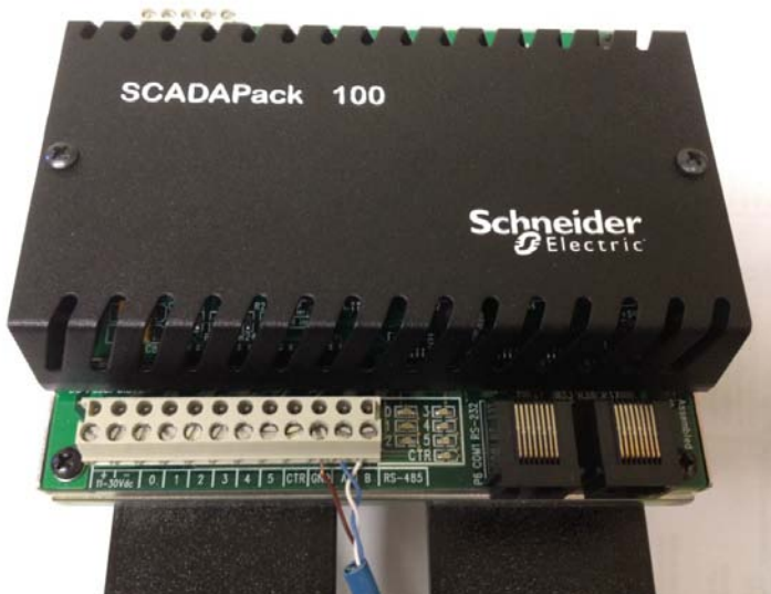
Figure 8 – SCADAPack 100 with CAT5E Cable Attached to COM1 (RS485 capable serial port)
