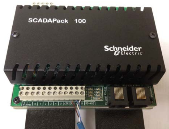
Figure 21 - SCADAPack 100 With Attached CAT5E Cable
